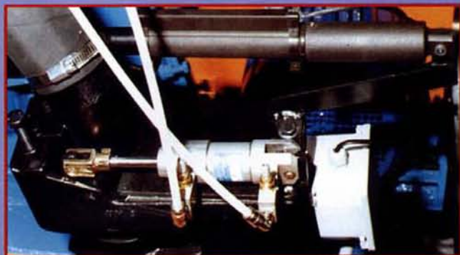
Abrasive gate arranged with remote control
